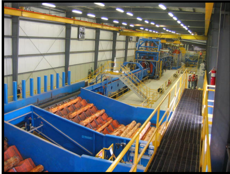
Wave Log Feeders and Full Line
